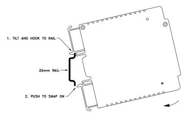
Figure 3.2 — Mounting on 35mm DIN Rail
